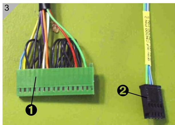
2. Connect plugs (1) and (2) to the USI board (fig. 4).
