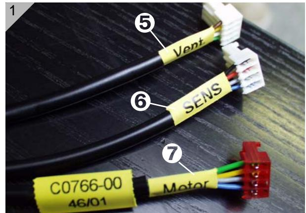
1. Connect the VENT (5) and SENS (6) cables, which are part of the cable harness, to the sockets on the PLC board that bear the same names (fig. 2).
