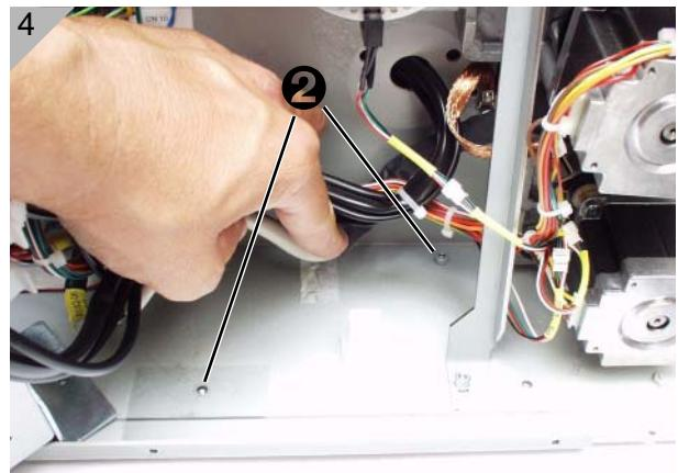
6. Pull at the wiring harness (3) as illustrated to make room for the insertion of the PLC module (fig. 5).
