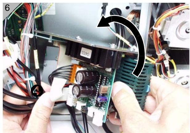
8. Right now is the best moment to connect the PLC module to the USI board!
