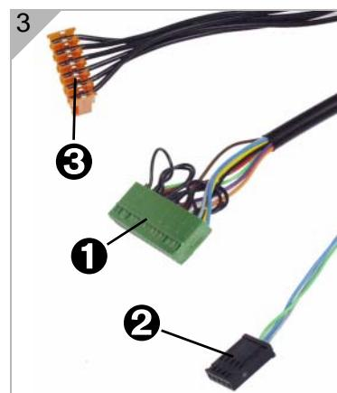
3. Connect the plugs (1) and (2) to the USI board (fig. 4).
