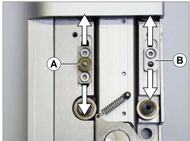
[10] Adjusting the home position. Remove the gaiter to get to those aluminium plates.
