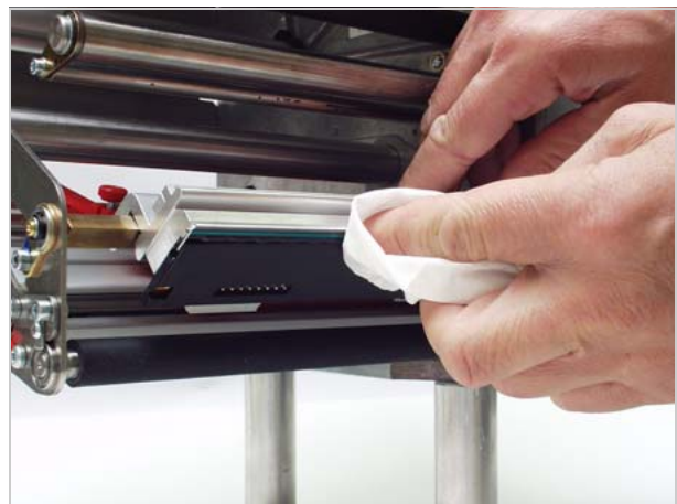
[60] Clean the printhead with alcohol.
