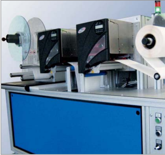
[6] Application with two PEM modules for two colour printing. Between the two modules is a buffer loop. At the left side, the printed material is wound up.
