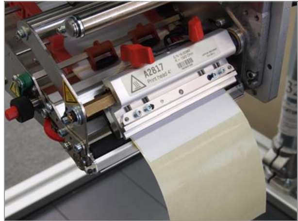
[36] Peel the labels off on a length of 50 cm.
