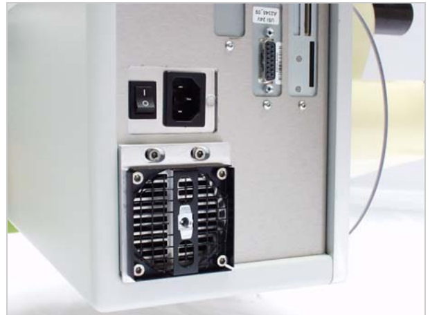
[79] Filter housing removed.
