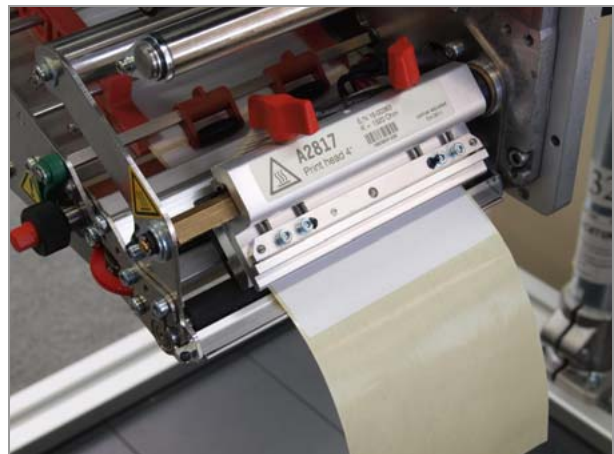
[41] Peel the labels off on a length of 50 cm.
