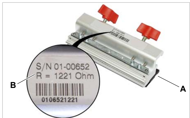
[68] Printhead (A) with resistance identification (B); in this case: 1221 Ohm.
