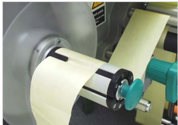
[49] Fastening the backing paper to the rewinder.
