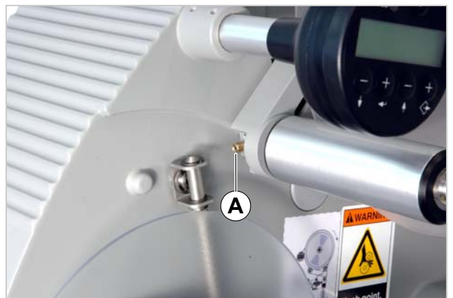
[54]] Setting screw (A) at the unwinder dancer arm.
