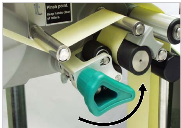
[48] Close the pressure roller.
