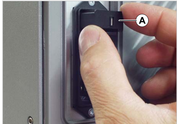
[47] Remove the fuse insert (A).
