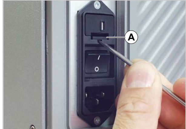
[46] Unlock the fuse insert.
