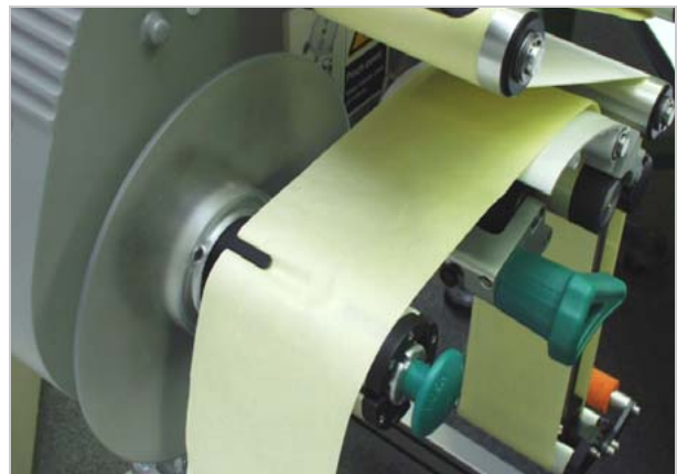
[35] Fastening the backing paper to the rewinder.
