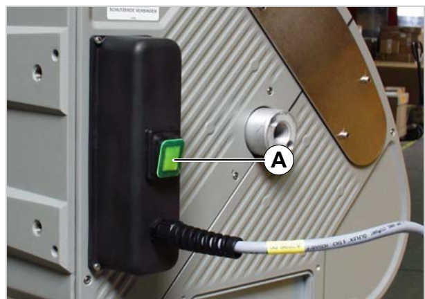
[42] Mains switch (A) of ALS 104 with dust/splash guard option.
