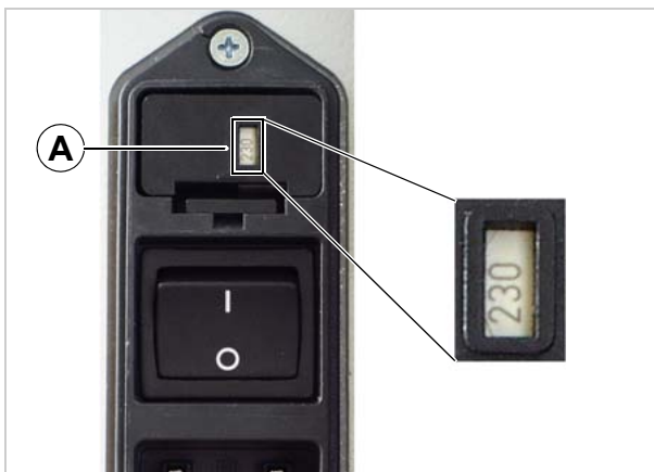
[23] Voltage display on the fuse insert (showing 230 V here).
